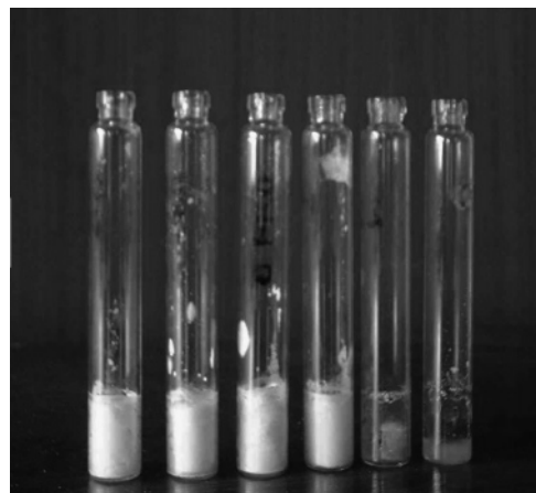
Figure 4. Picture of the PVP-40 matrix samples with maximum degree of collapse ( D_{c,max} ) at several RHs at 25 °C.
